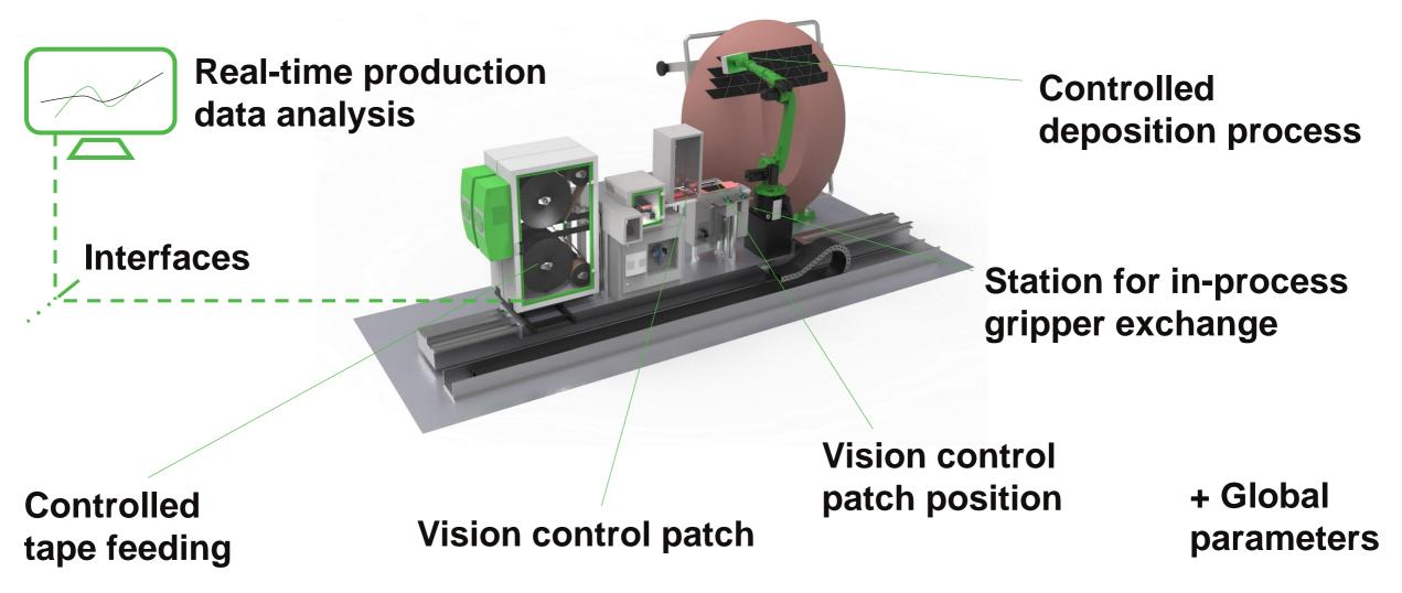
Objective: Replace individual unit tests by continuous process monitoring
